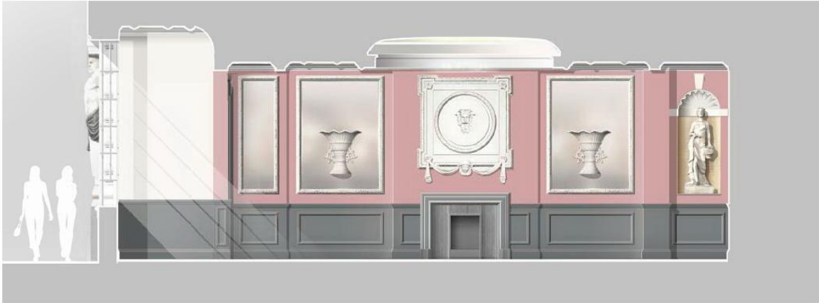
① PROPOSED GROUND FLOOR FACADE SECTION + INTERNAL ELEVATION OF WESTERN WALL (RETAINED INSITU) NTS
